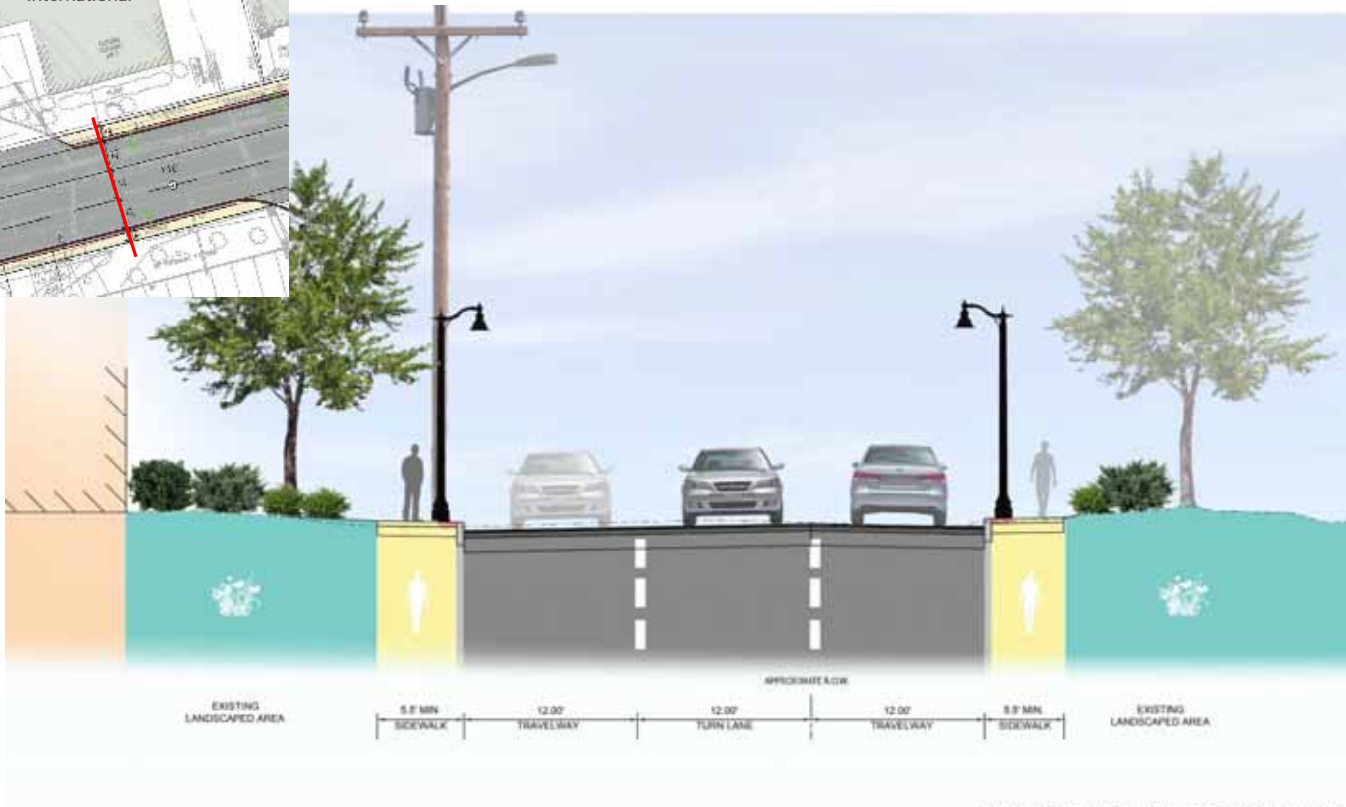
CONSTRAINED SECTION- 12' CENTER TURN LANE
